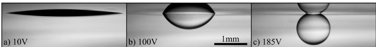
Figure 1. Experimental images of the contact change in response to voltage of a thick low dielectric liquid film.
