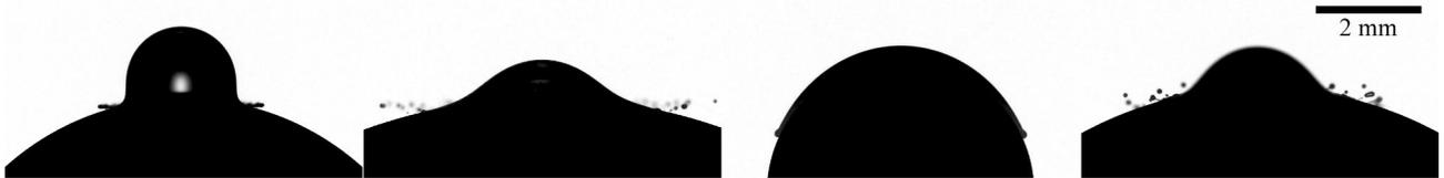
Figure 1: Examples of various impact outcomes for droplets on spheres, from deposition to splashing. Sphere diameters of 5 mm–20 mm are shown. Times after impact {0.2, 0.6, 1.0, 0.4} ms for each frame, respectively.
