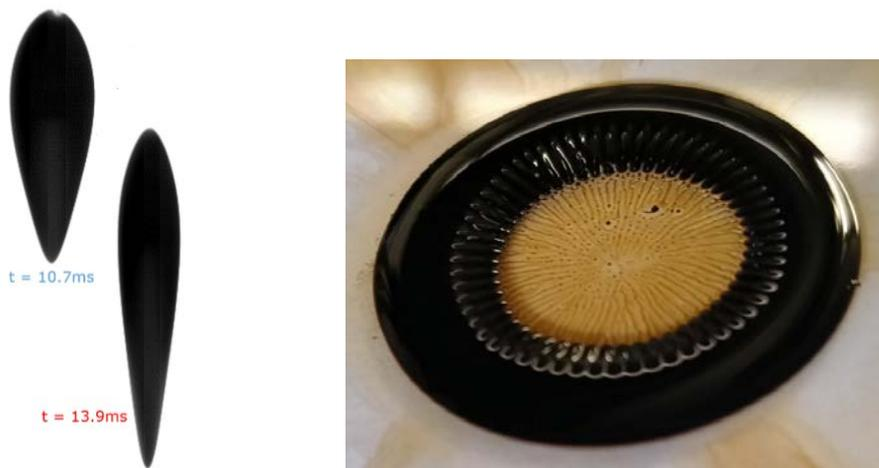
Figure: Left, ferrofluid drop profiles prior to drop impact on a glass slide placed above a bar magnet, labelled with relative time elapsed, and (right) a drop following impact.
