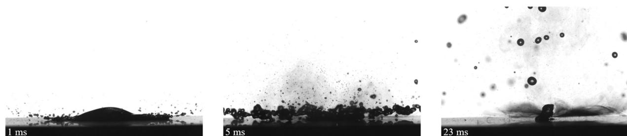
Figure 1: Characteristic behavior of droplet impact on porous heated surfaces in the *partial rebound with breakup* regime.
