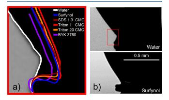
**Figure 4.** Droplet free surface near the contact line, 0.2 ms after impact. (a) Profiles after impact on Teflon at  $U_0 = (1.20 \pm 0.06)$  m s<sup>-1</sup>, overlaid onto a photo of water, where the contact line speed is  $u_{cl} = (5.54 \pm 0.25)$  m s<sup>-1</sup>. (b) Photos in the vicinity of the contact line for water (top) and Surfynol (bottom).
