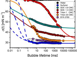
**Figure 2.** Dynamic surface tension for water and all surfactant solutions used in this work. Symbols indicate average data as measured by the maximum bubble-pressure tensiometer, for which error bars represent either 3 times the standard deviation or the largest difference observed by varying the critical point. Lines represent eq 2 applied to the data, either by a least-squares fit to the rapid fall region via eq 3 (solid lines) or manual fitting (dashed lines).
