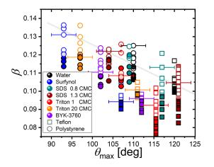
**Figure 6.** Splashing for droplets containing surfactants impacting polystyrene and Teflon. The plot shows the splashing parameter  $\beta$  in terms of  $\theta_{max}$ . Here, splashing is denoted by open symbols, while closed symbols represent no splashing. Representative error bars are shown for some data points for simplicity; vertical error bars are much smaller than the size of the symbol.
