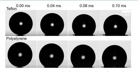
**Figure 5.** Near-identical Triton 1 CMC droplets impacting Teflon (top) and polystyrene (bottom) at  $U_0 = (3.07 \pm 0.02)$  m s<sup>-1</sup>. Splashing is observed for the impact on Teflon, while no secondary droplets emerge after the impact on polystyrene. This result indicates that substrate wettability via the dynamic contact angle influences the splashing behavior of surfactant-laden droplets, similar to simple fluids.
