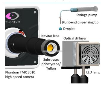
**Figure 1.** Schematic view of the experimental setup used to visualize the impact of droplets. Various systems were used in this work; the figure shows an example using a Phantom TMX 5010 high-speed camera equipped with a Navitar lens and lighting provided by a 100 W LED.
