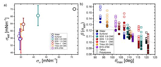
**Figure 8.** (a) Predicted prevailing surface tension  $\sigma_{est}$  at the onset of splashing in terms of the equilibrium surface tension  $\sigma_0$ . The prevailing value  $\sigma_{est}$  is calculated such that the splashing threshold of each surfactant matches that of eq 4. In all cases  $\sigma_{\infty} < \sigma_{est} < \sigma_0$ . (b) Reconstruction of Figure 6: The  $\beta$  value has been calculated by employing  $\sigma_{est}$  (surface tension at the onset of splashing) in eq 1.
